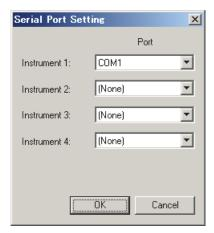
When two or more CM-700d/600d units are connected, the specular component mode (SCI, SCE, or SCI+SCE) and measurement area (SAV (3 mm) and MAV (8 mm)) specified for the first-connected instrument (instrument 1) are applied to the other connected instrument(s).
