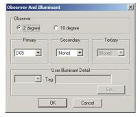
Only one pair of observer and illuminant can be specified for each document file. This setting does not affect the observer and illuminant that have been specified with the instrument.
