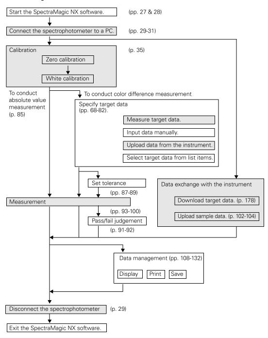
The shaded sections indicate functions available only when the spectrophotometer is connected and the protection key is attached to the computer.
