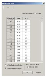
Sample display when the CM-2600d/2500d is connected
