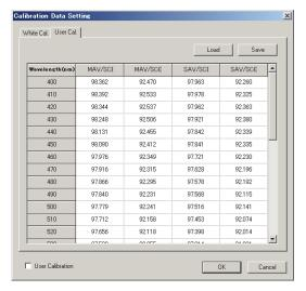
Sample display when the CM-700d/600d is connected The User Calibration check box and the User Cal. tab are supported by the SpectraMagic NX Professional Edition only.
