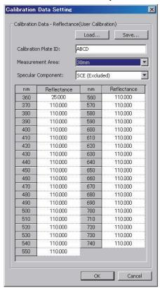
**2-3.** Set the calibration value by entering spectral reflectance or spectral absorbance. Or, click the Load button to load the existing calibration value file and set the value.
