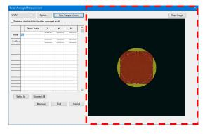
When the CM-36dG, CM-36dGV, or CM-36d is connected, the Sample Viewer panel (indicated by red dotted-line rectangle above) will be shown when Show Sample Viewer has been clicked.
