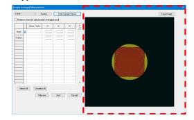
When the CM-36dG, CM-36dGV, or CM-36d is connected, clicking Show Sample Viewer will open the Sample Viewer panel (indicated by red dotted-line rectangle above) showing a real-time view of the measurement subject from inside the instrument to help in accurately positioning the subject. Clicking Hide Sample Viewer will hide the Sample Viewer panel.
