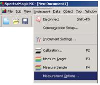
The interval measurement repeats measurement a specified number of times at specified intervals. The measured sample data is received after every measurement.
