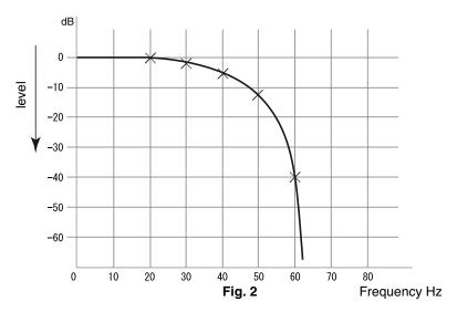
From this, it is possible that even if a flicker of a large amplitude and frequency of 60 Hz or higher exists the human eye cannot recognize it as a flicker.
