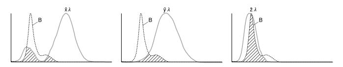
Fig. 4 Outputs of Sensors  $\overline{x}\lambda$ ,  $\overline{y}\lambda$ , and  $\overline{z}\lambda$  by Emitted Monochrome Light B
