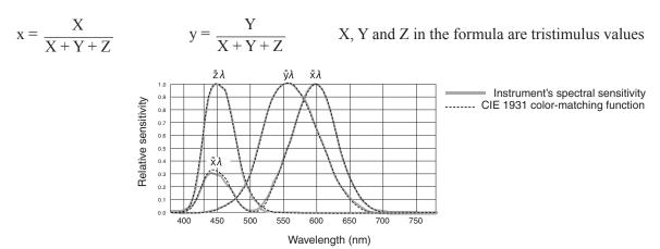
Fig. 1 Instrument's Spectral Sensitivity
