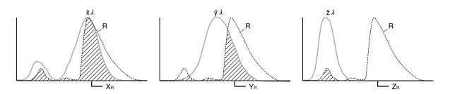
Fig. 2 Outputs of Sensors  $\overline{x}\lambda$ ,  $\overline{y}\lambda$ , and  $\overline{z}\lambda$  by Emitted Monochrome Light R
