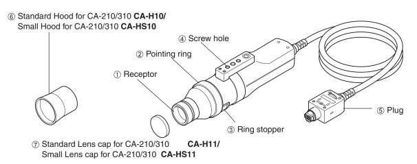
Measuring is done with the probe in close contact with the surface of display in the measuring part of this equipment. There are 2 m(6.6ft.) and 5 m(16.4ft) long cords. There are 4 types of Measuring Probes.
