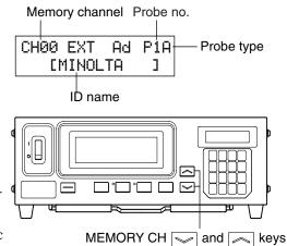
The desired memory channel can be selected by switching from one to another by pressing the MEMORY CH  $| \searrow |$  and  $| \searrow |$  keys.
