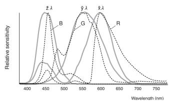
Fig. 1 Display's Spectral Distribution and Sensor's Spectral Sensitivity
