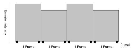
Fig. 6 Emission status of LCD with "Flicker"
