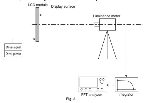
Fig. 3 shows that the output signal (Fig. 1) from the luminance meter (used to measure the LCD) is guided to the integrator.
