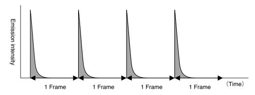
Fig. 5-1 Emission characteristics of CRT
