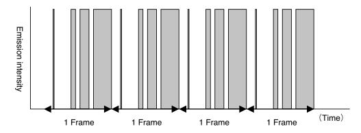
Fig. 5-2. Emission Characteristics of PDP
