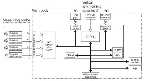
Fig. 2 Measurement Block Diagram
