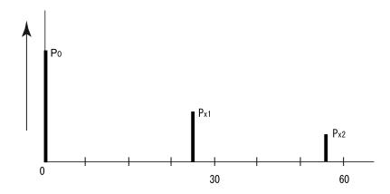
As shown in Fig. 4, when two or more frequency components (P0, Px1, Px2) exist, the maximum value among all the frequency components (Px1, Px2 in the case of Fig. 4) except for P0, that is the component of frequency 0, will be set as Px. With the JEITA method, the flicker amount in this example is calculated by the following formula.
