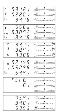
3 Analog display section ...... Displays the difference (%) between the measured value and the target color or the difference (%) between measured values.
