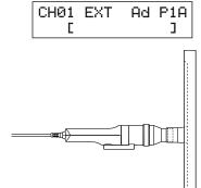
3. Place the measuring probe against the display.
