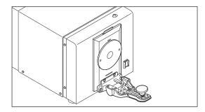
2. Fit the projections of the zero calibration box into the grooves on the CM-3700A-U and then close the sample holder to hold the box in place.
