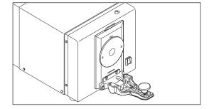
2. Position the white calibration plate so that it is held in place by the sample holder by fitting the sample holder pad into the concave (rear) side of the white calibration plate as shown at right.
