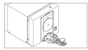
2. Remove the currently attached target mask by pulling it toward you.
