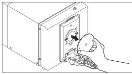
3. Align the target mask positioning holes of the target mask to be attached with the target mask positioning pins of the Spectrophotometer's specimen port baseplate and slide the target mask in against the specimen port baseplate.
