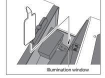
3 Close the transmittance specimen chamber cover.
