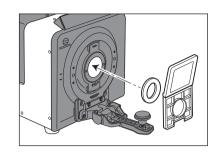
For fluorescence measurement that does not require strict accuracy (fluorescence calibration is not performed), perform measurement with the UV cutoff filter not covering the xenon lamp (with UV output at 99.9). When the below setup is completed, execute 100% calibration from the software.
