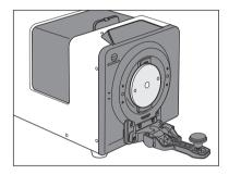
2 Fit the protrusion on the zero calibration box into the indentation on the instrument, and then hold this box in place with the sample holder.
