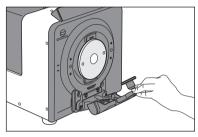
2 Pull the currently installed target mask or protective cap toward you to remove it.
