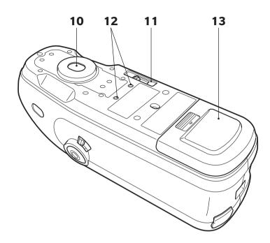
10 Specimen measuring port This is the aperture for measuring samples.
