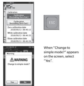
Set "Simple mode" under <Setting> - <Instrument Mode>.
