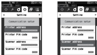
2 Enter the address of the Bluetooth device to be connected.
