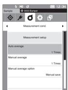
2 Use [▲] or [▼] to move the cursor to "Measurement setup", and then press the [Confirmation] key. The <Measurement setup> screen is displayed.
