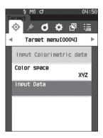
2 Use [▲] or [▼] to move the cursor to the item to set, and then press the [Confirmation] key. The <Input data> screen is displayed.
