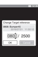
Notes If a number to which no color difference target data has been set, the target will be determined as "None" and the color difference and pass/fail judgment will not be displayed.
