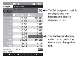
"FAIL" is printed in the print output, and "x" is appended after any value that exceeds the tolerance. Pass/Fail screen
