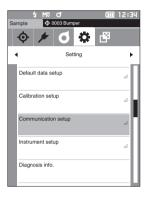
2 Use [▲] or [▼] to move the cursor to "Communication setup", and then press the [Confirmation] key. The <Communication setup> screen is displayed.
