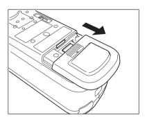
3 Rotate the battery retainer and insert the lithium-ion battery. (Follow the indications in the battery compartment to avoid confusing the battery polarity.)
