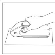
To measure concave surfaces, as shown in the following figure, use the standard flat type battery cover (CM-A218).
