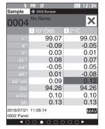
Memo/ • When the number of sample data sets stored in the memory reaches 7,500, "The device memory is full. Please delete some data to measure." will be displayed, indicating that some data sets must be deleted before measurement is possible.
