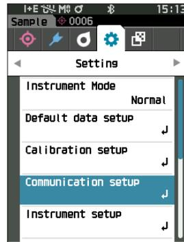
**2** Use [▲] or [▼] to move the cursor to "Communication setup", and then press the [Confirmation] key.
