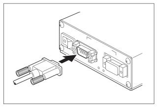
Plug the other end of the RS-232C cable to the serial port (COM port) on the computer. The procedure is now complete.
