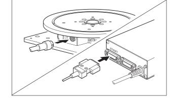
Plug one end of the RS-232C cable to the control box.
