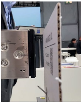
High-gap printing enables clear character printing even if the surface of a corrugated fiberboard is uneven.
