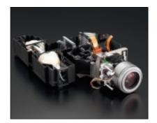
This optical unit with a twin lamp system realizes extremely bright images for LCD projectors.
