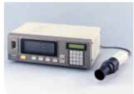
CA-210 The CA series of color analyzers, which measure light source color, are used to measure the color and luminance of LCDs and cathode-ray tubes (CRTs).
